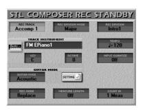
(2) Press the TRACK field and use the DATA/ENTRY dial to select the track you wish to assign another sound (or Drum Set) to.
